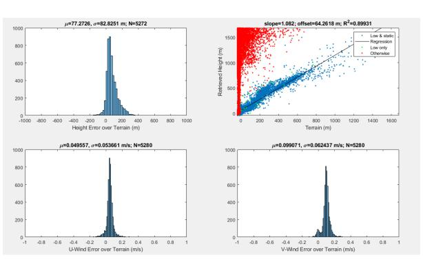
**Figure 5.** Comparison of ground point NOAA-20 VIIRS (I1 band)/GOES-16 ABI (band 2) stereo winds retrievals (14 Nov. 2020 18:36Z) against known terrain height (from elevation model) and expected (ie., zero) wind speed.
