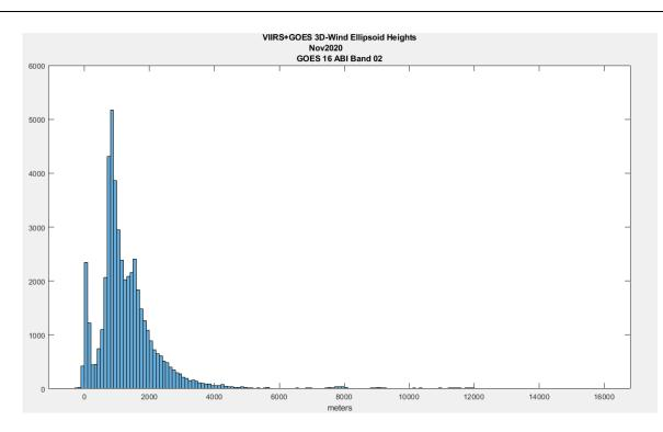
Figure 4. Histogram of the retrieved wind ellipsoid height (m) shown in Figure 2.
