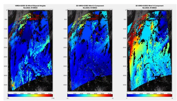
**Figure 2.** Retrieved NOAA-20 VIIRS (I1 band)/GOES-16 ABI (band 2) stereo ellipsoid heights (left), wind u-component (center), and wind v-component (right) valid on 14 Nov. 2020 18:36Z
